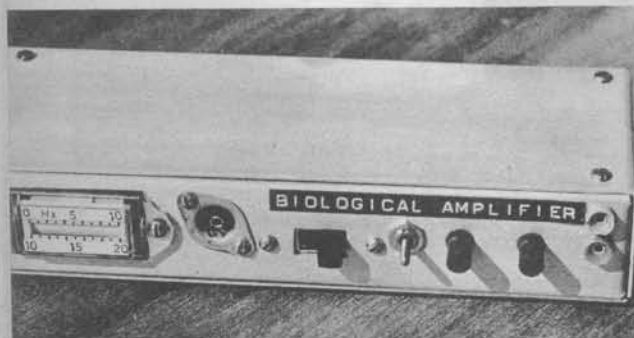
Brain rhythm frequency meter. The coaxial socket provides a connection to the visual feedback unit
