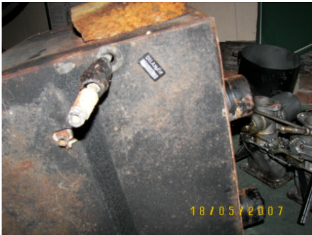
The 420 evaporator case – note the gasket for direct seal against the underneath of the parcel shelf and the Delanair decal.
