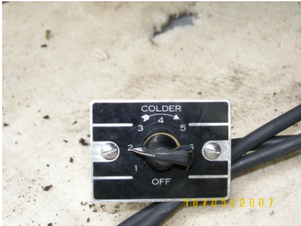
A fascia mount temperature control with long sensor probe
