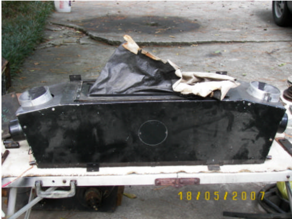
The S-type / MK2 evaporator case – note the shape to fit the boot space. The round ducts for the air are clearly seen, as is the remnant of the cloth duct for air return.
