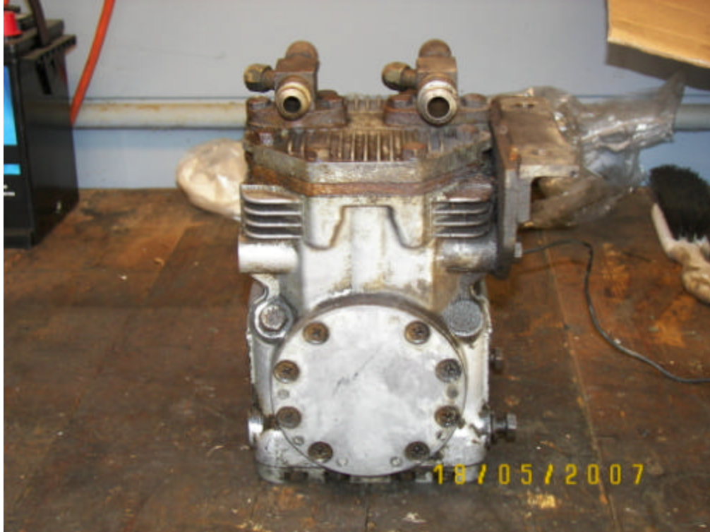
The earliest York A209 found on a Jaguar by the Author. It is a 1956 model (note the “retro” fin look – no doubt thought at the time to be needed for cooling).
