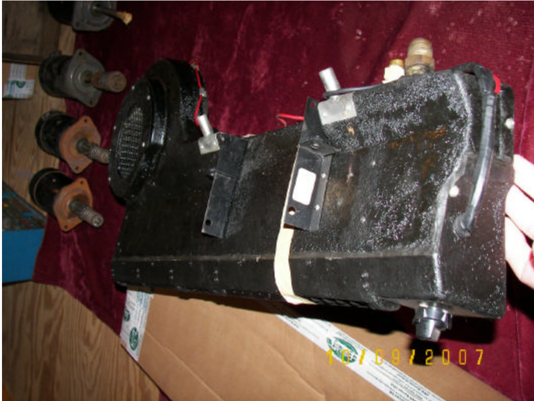
Radio mounts on an E-type evaporator case – note the serial number sticker on the rear bracket
