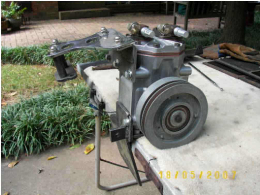
A York A209 compressor for a MK2 / S-type with mounting hardware. Note the bracket is chromed where it would cross the polished cam cover.
