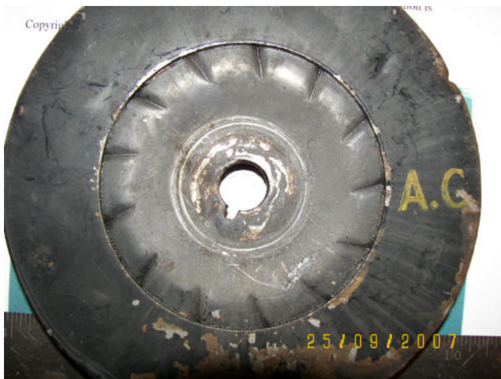
An E-type air conditioning Alternator Fan - the "A.C." designates this as a reverse unit for use only when air conditioning is fitted
