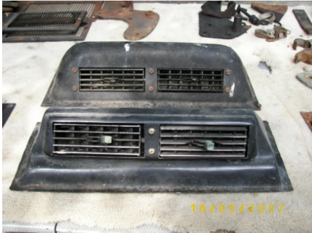
MK 10 air vent (top later metal – bottom early plastic)
