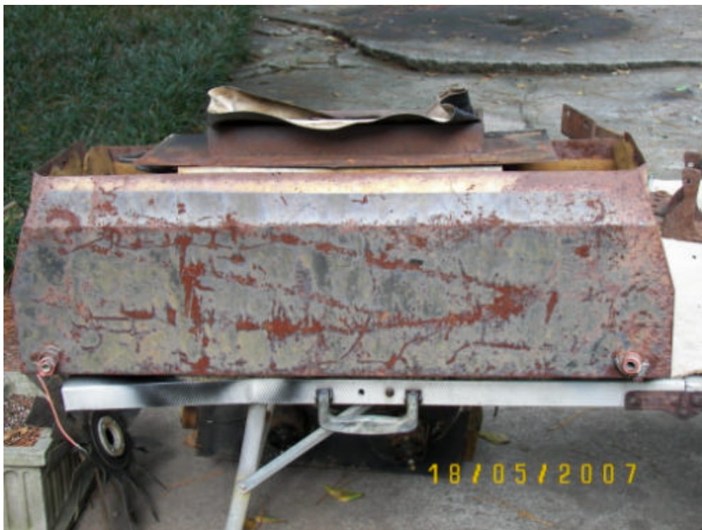
The evaporator case removed from a MK VII M. It has an unusual coffin shape – the remnants of the Jaguar decal were there, but not visible in the photo
