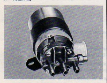
Check 2-pole plug for corrosion and replace where necessary.
