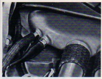
Temperature sensor I is installed in the top of the intake manifold.
