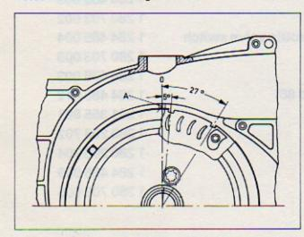
A = notch in cooling blower housing
