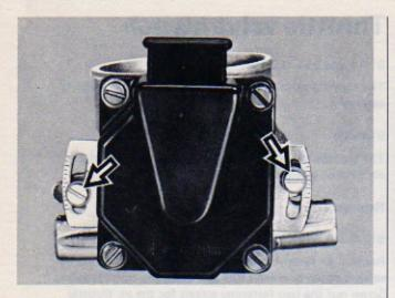
Throttle valve switch 0 280 120 021 as from FD 323 Throttle valve switch 0 280 120 032 as from FD 321
