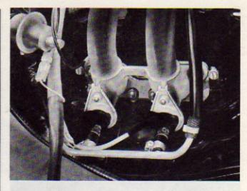
Installation of the injection valves
