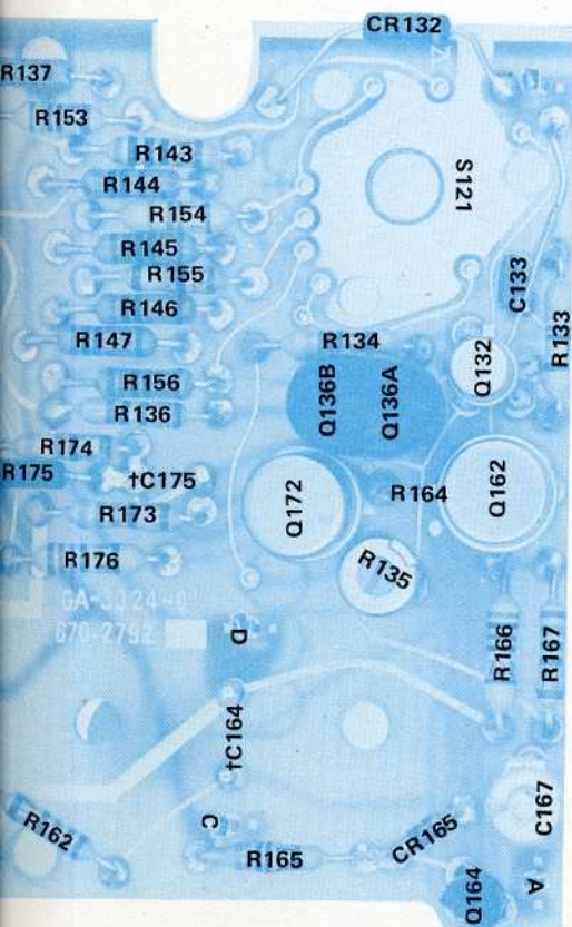
Fig. 9-4 A2—Preamplifier circuit board
